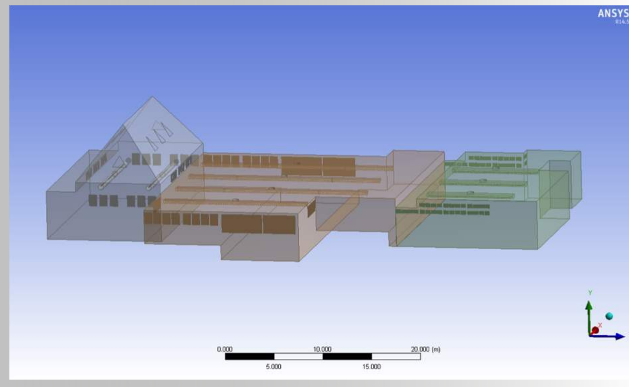
10.1 Volume of fluid (air) to be affected by the system is modeled
